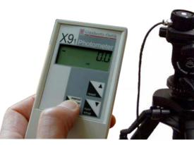
diagnostics for example. For this reason current DIN and EN regulations specify that light meters must have a maximum permissible error  $f_{tot}$  of ±10%. According to DIN-5032 Part 7 these are regarded as DIN class B instruments. This quality designation is necessary because class C instruments - incidentally many photometers on the market are not certified at all - that are used to measure different types of light sources such as standard illuminant A incandescent lamps,
